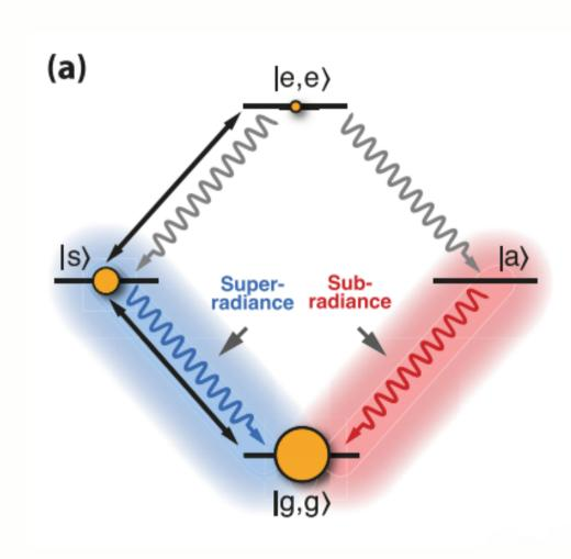
Level scheme of the two-ion system in the Dicke basis[S. Richter et al., 2023]
